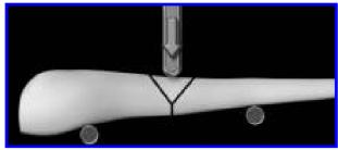
Figure 2—Illustration of biomechanical testing of an equine MTII and MTIV in 3-point bending. Peak load to failure (N) and area at the site of failure (mm²) were recorded. Peak stress to failure (N/mm²) was calculated.
